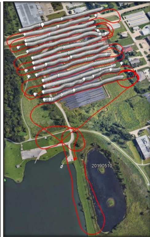
Figure 30. Flight path & photo locations for 2019 May 10
