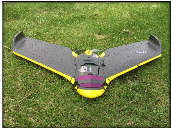
Figure 7. eBee unmanned aerial vehicle
