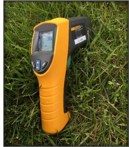
Figure 11. Fluke 561 IR thermometer
