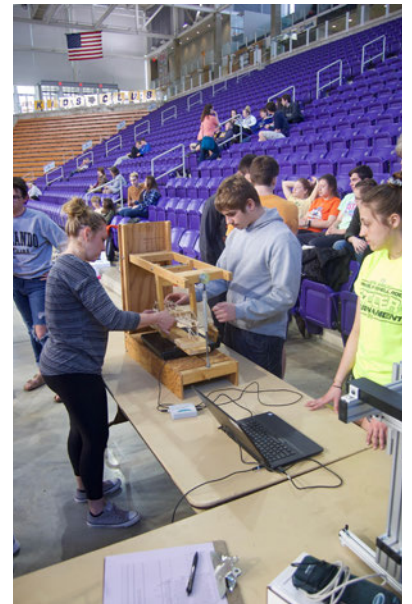
Student positions a toothpick bridge on the bridge tester, which will test its strength, often to destruction.
