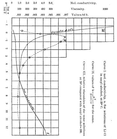
number of grams of Li Cl per litre, M = molecular weight of Li Cl = 42.37, we have  $m = M(\frac{1}{2})^p$ , in which p is the desired convenient measure of the dilution.
