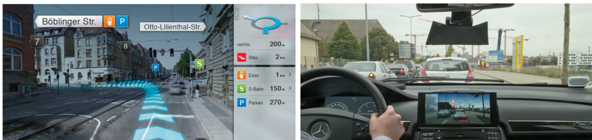
Figure 1: Concept art and prototype of vehicular AR-System. Navigation directions, street names and house numbers as well as POIs are shown
