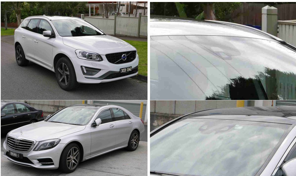
Figure 5: Examples of forward facing camera packages in automobiles. Top row: Volvo XC60 (1st generation). Bottom row: Mercedes-Benz S-Class (W222)
