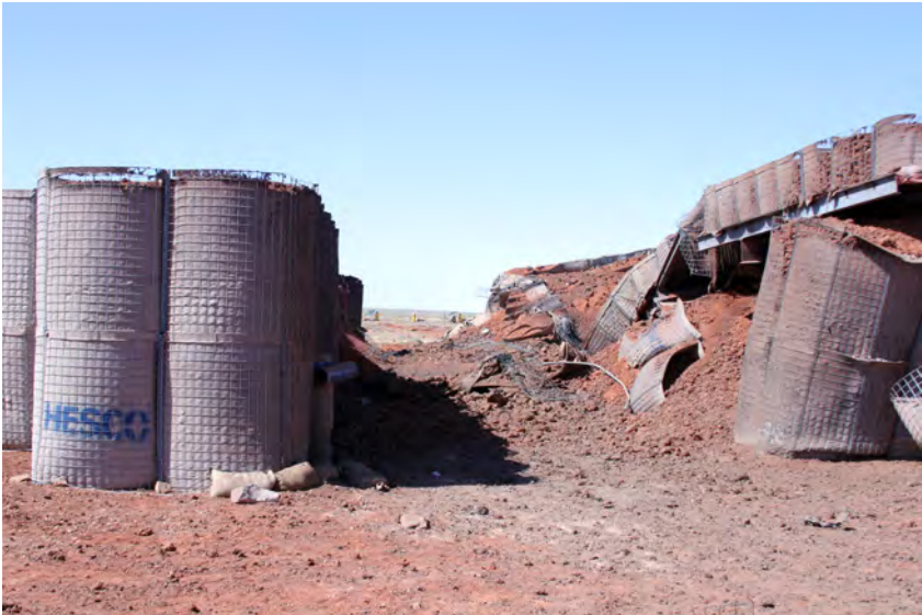
Figure 19 – Container-Based Barricade Demonstrated in a Large-Scale Explosive Storage Trial. 91)
