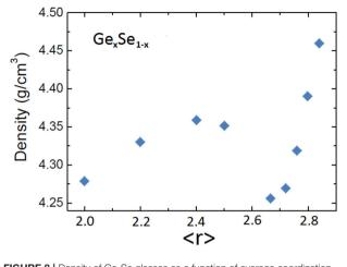
**FIGURE 8** | Density of Ge-Se glasses as a function of average coordination <*r>*. Data from Yang et al. (2013).
