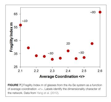
being the strongest and 0D molecular glasses such as o-terphenyl being the most fragile (Angell, 1991). In the case of  $As_2Se_3$  the sheet structure where layers are only bonded by weak Van der Wall interactions leads to faster collapse of the structure with temperature and a more fragile behavior. Hence, in the case of the As-Se system, dimensionality eventually dominates the fragility behavior.
