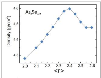
**FIGURE 6** | Density of As-Se glasses as a function of average coordination <*r>*. Data from Yang et al. (2010).
