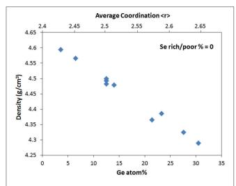
**FIGURE 2** Density of Ge-As-Se glasses with stoichiometric composition (Se rich/poor = 0) as a function of percentage of Ge atoms and average coordination <*r*>. The density varies linearly with Ge% when the effect of stoichiometry is neutralized.
