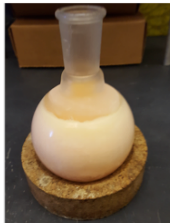
"Shell Freezing" 12 hours to sublimate
