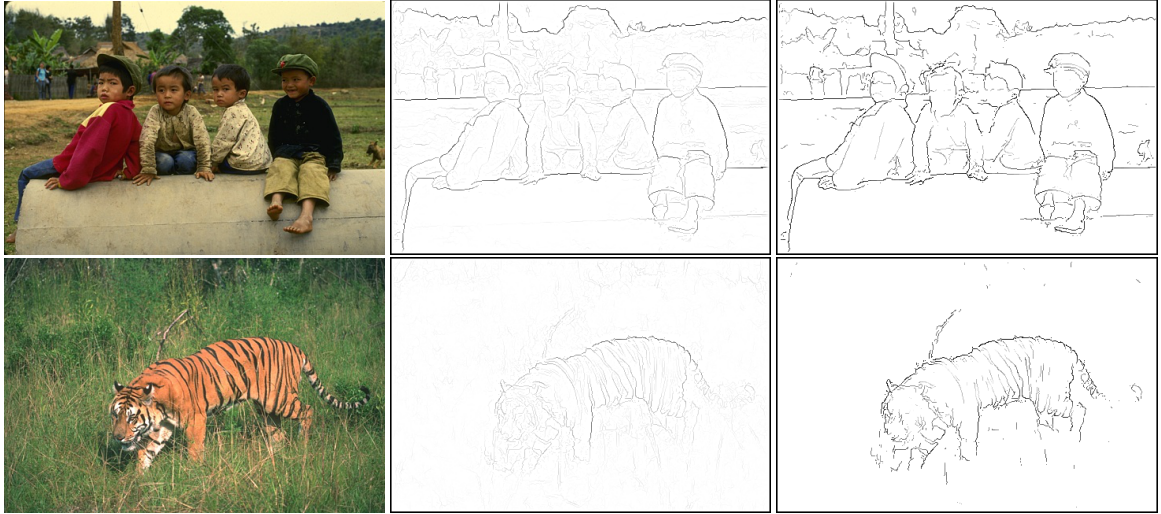
Figure 10: Qualitative results on the BSDS benchmark. The first column of images represent input images. The second column illustrates SE [15], while the third column depicts HfL boundaries. Notice that SE boundaries are predicted with low confidence if there is no significant change in color between the object and the background. Instead, because our model is defined in terms of object-level features, it can predict object boundaries with high confidence even if there is no significant color variation in the scene.
