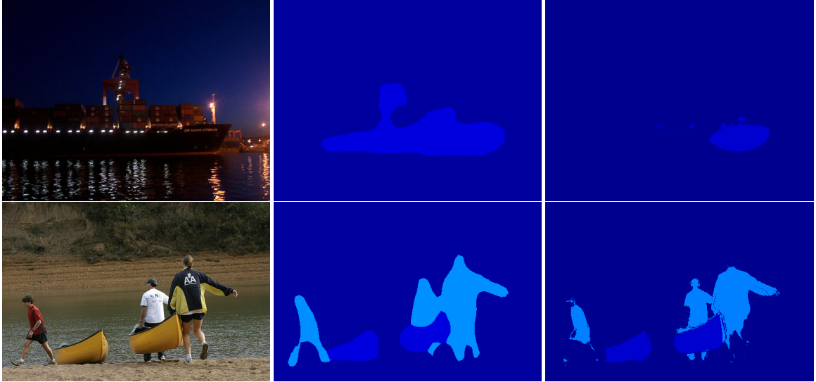
Figure 15: Examples illustrating shortcomings of prior semantic segmentation methods: the second column shows results obtained with a FCN [27], while the third column shows the output of a Dense-CRF applied to FCN predictions [28, 29]. Segments produced by FCN are blob-like and are poorly localized around object boundaries. Dense-CRF produces spatially disjoint object segments due to the use of a color-based pixel affinity function that is unable to measure semantic similarity between pixels.
