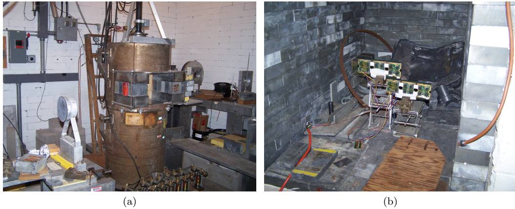
Figure 4.3: (a) The cobalt-60 source and (b) TRT endcap triplet boards, about 3 meters away from the source.
