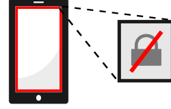
(c) The phone displaying visual indicators that it is providing the Low personality: domain = \text{LOW} , and source is classified Low to reflect that we trust the user not to type in secrets.
