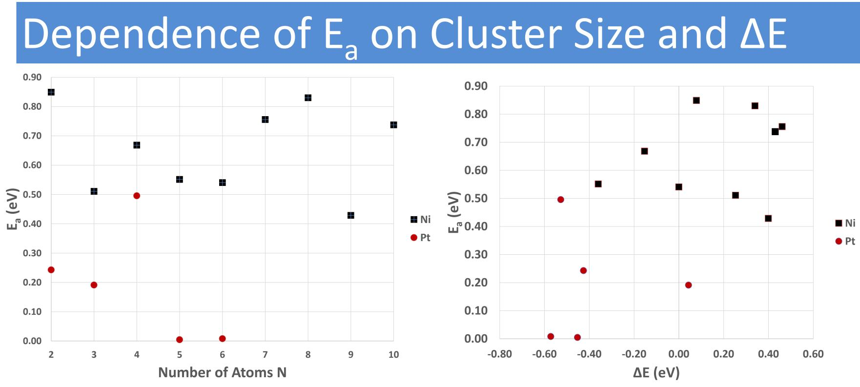
E<sub>a</sub> varies according to cluster size, but not in a linear fashion No linear relation between  $E_{a}$  and  $\Delta E$ ; Bell-Evans-Polanyi (BEP) principle does not hold for these results
