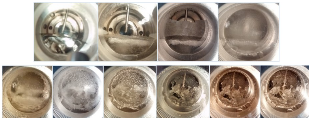
Figure 3.4: Top panel: Visual observation of the evolution of the different phases during gas hydrate crystallization (from left to right: directly after water injection; after stirrer has been set to 400 rpm; 1 min after the gas hydrate formation incipient; 48 min after the gas hydrate formation incipient). Bottom panel: Visual state of the system during the gas exchange process (from left to right: t= 0h ; t= 1.47h ; t= 18.90h ; t= 89.73h ; t= 118.90h ; t= 145.73h ).
