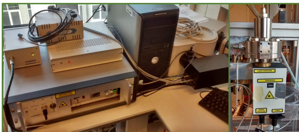
Figure 4.6: Raman spectrometer connected to the apparatus for fluid analysis. Analytical section (Left), and high-pressure windowed side and optical head (Right).
