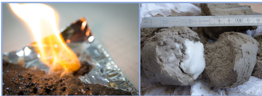
Figure 1.3: Left: combustion after ignition of muddy thermogenic gas hydrates sampled in the Sea of Marmara with a 12 m gravity core, at a depth around 658 m and a seafloor temperature of 287.15 K (L.N. Legoix, 2014). Right: Methane hydrate lens formed in laboratory with a clay/sand mixture (modified from Ruffine [2015]).
