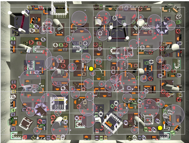
Fig. 4. In this top-down view of the Tradeshow scene with 200 sources, clustering has been done for listener L_1 . Clustering at listener L_1 produces 95 clusters (2.1x reduction in number of sources), while clustering at listener L_2 produces 52 clusters (3.8x reduction), since the clustering can be more aggressive. The size of nodes in the octree used to accelerate clustering increases with the distance from the listener.
