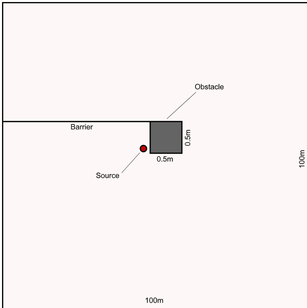
Fig. 1. The figure shows the setting used for characterizing diffraction. The obstacle was 0.5m x 0.5m. The solid barrier prevents the sound from reaching the listener from behind the obstacle. The barrier and the obstacle are fully absorptive to prevent any reflections and making sure only the diffracted sound reached the listener. The figure is not drawn to scale for better viewing of the experimental setup.
