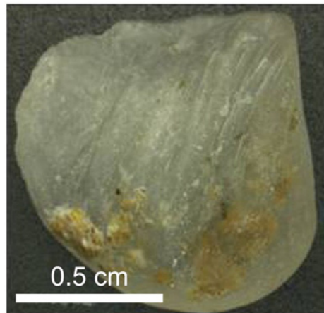
Figure 2.9: Image of an ASR gel fragment collected from the Furnas dam [1]
