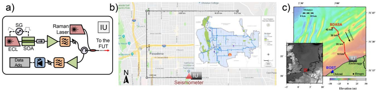
Figure 1. (a) Setup of the CP- \phi OTDR employed for the experimental tests. ECL: External cavity laser, SG: Signal generator, SOA: semiconductor optical amplifier, FUT: fiber under test, IU: Interrogator unit. (b) Geometrical distribution of the fiber in Pasadena, including the location of the reference seismometer, the interrogator unit, and an inset with the real distribution of the fiber over the city. (c) Map of the fiber distribution in the cost of Zeebrugge, including the location of the seismometer (BOST), the interrogator unit, and an inset with the location of the fiber over the north shore of Europe.
