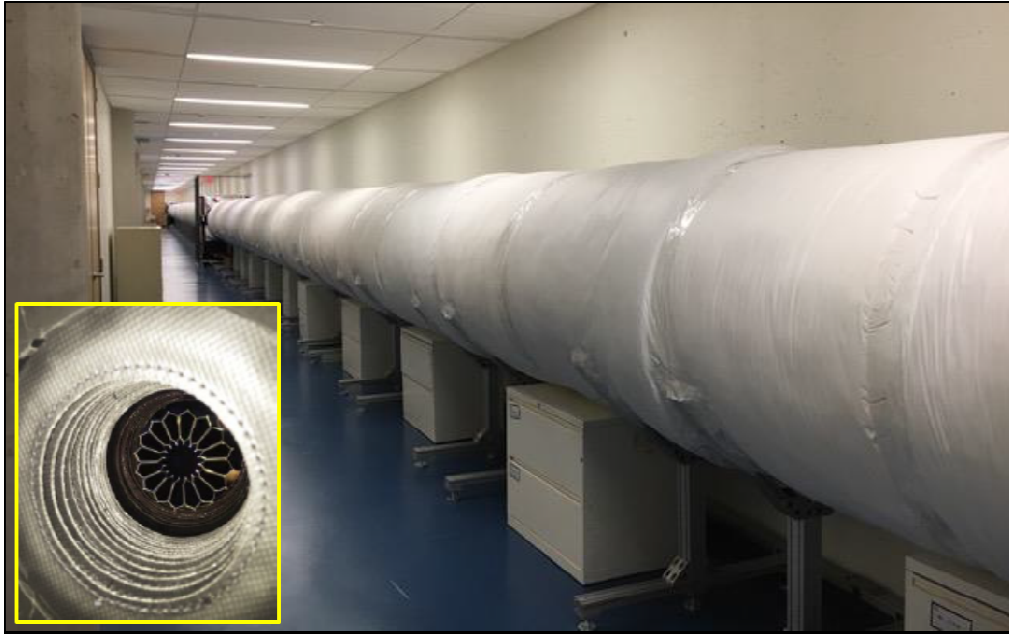
Figure 11. S5's starshade model validation testbed at Princeton. Model starshade shown in inset.
