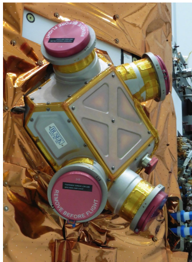
Figure 14. A single cluster of four Busek Co. CMTs integrated on the LISA Pathfinder Spacecraft just prior to launch. Image courtesy ESA / Airbus.
