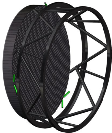
Figure 1. Baseline 4 m × 40 cm thick flat-back open-back isogrid core Zerodur mirror.
