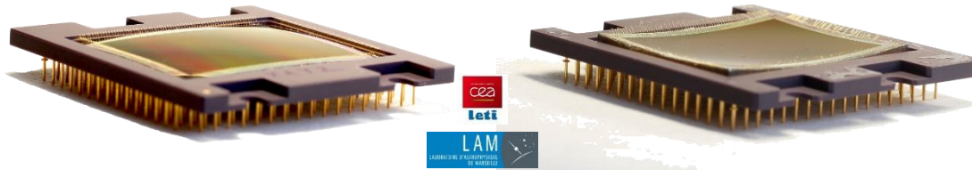
Figure 1: Convex and Concave curved VIS CMOS (28mmx32mm, 20 Megapixels, curved down to a radius of 150mm), fully functional. The exquisite performance of the curved sensors is described in Chambion et al, SPIE Photonics West 2018.
