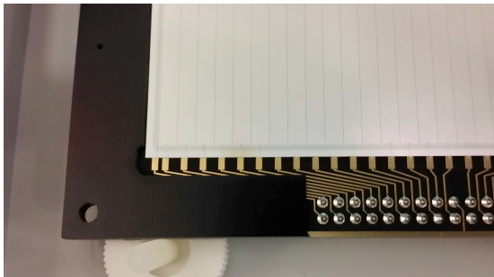
Figure 2: The strip side of a corner of an SSD mounted on its window-pane board (from Ref. [7]).
