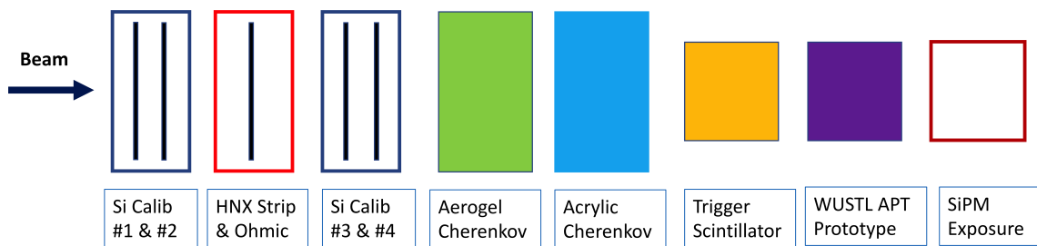
Figure 3: A schematic of the CERN test beam experimental setup used to determine the silicon detector charge resolution performance.
