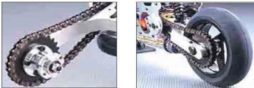
Rear wheel chain drive of a motorcycle
