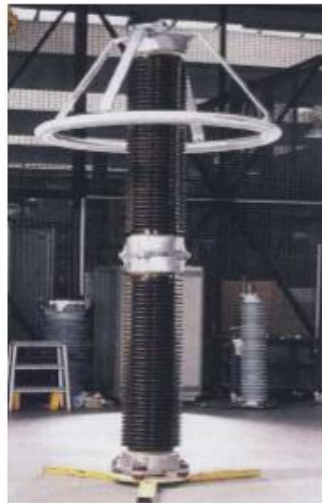
Gambar 2.13. Arrester (Sumber: https://lightningsource.wordpress.com )
