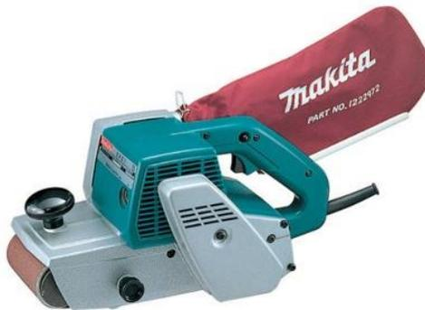
Gambar 4.30. Mesin Ampelas Type Belt Sander
