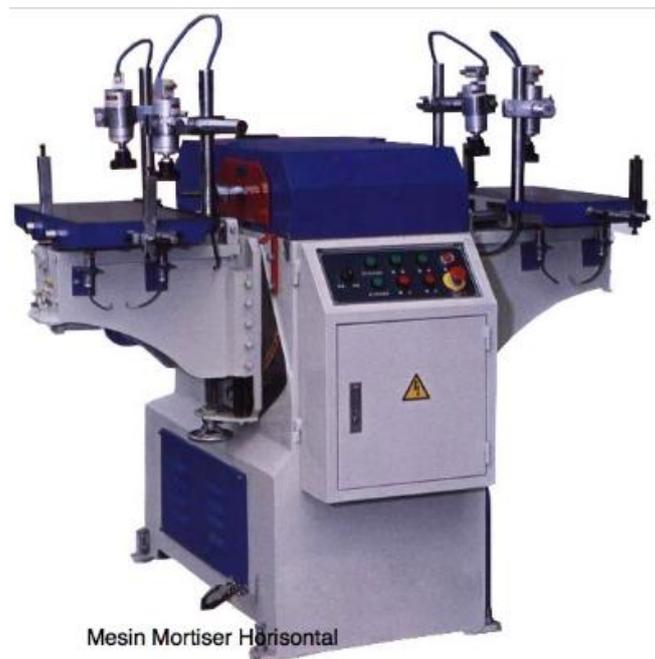
Gambar 5.13. Contoh Mesin Mortiser Horizontal
