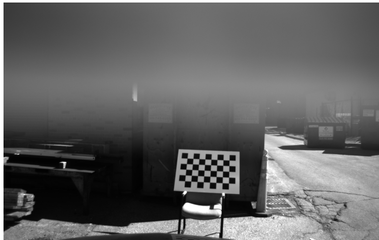
Figure 7.15: Cropped Camera Image from Hand-Eye Calibration Between Camera and Navigation System
