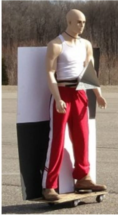
Figure 7.13: Calibration Target for Joint Calibration of Radar, LIDAR, and Mobileye Sensors
