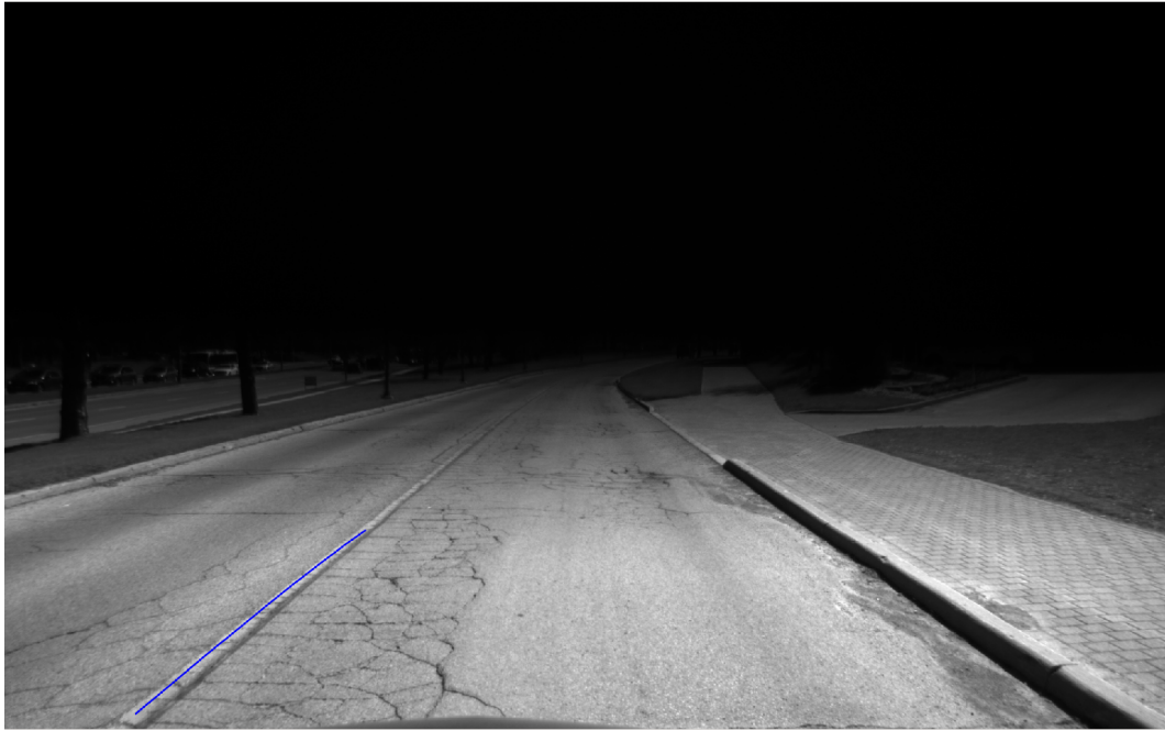
Figure 6.5: Polynomial Lane Model Fit Results on Original Image
