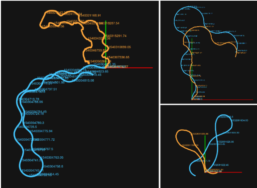
Figure 7.17: GPS (blue) and LIDAR Odometry (orange) for Various Calibration Maneuvers
