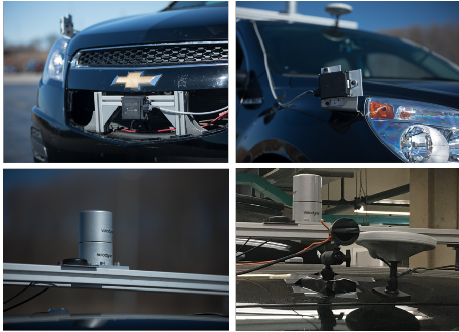
Figure 7.6: Installation View of Sensors with Front and Side Radar (top left), Side Radar and GPS Antenna (top right), LIDAR (bottom left), and Camera (bottom right)
