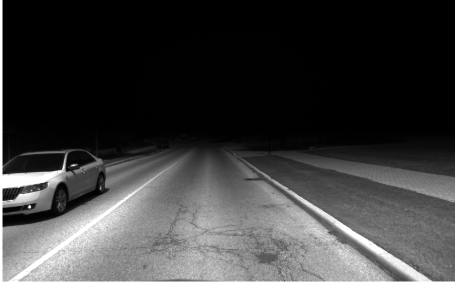
Figure 8.2: Improvement of Image with Tape Blocking Undesired Light Artifacts
