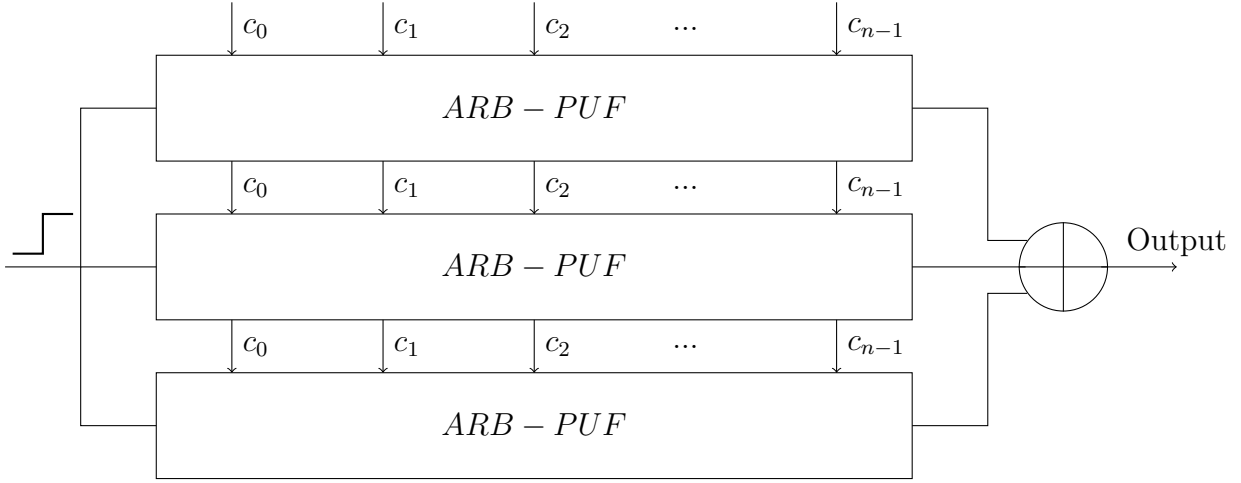
Figure 2.2: The XOR-PUF has 3 ARB-PUFs, accepting same challenge.
