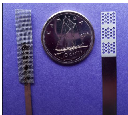
Figure 2.30 SPME-TM meshes: “wire-mesh” design represented on the left and “sheet-mesh” represented on the right.
