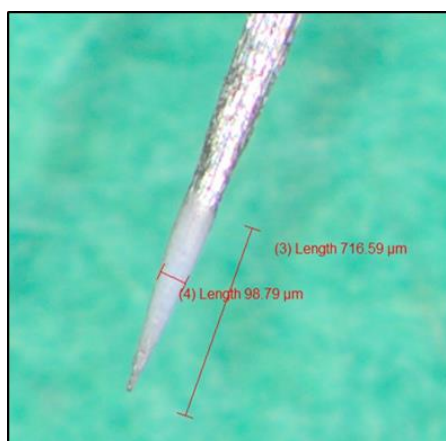
Figure 3.11 SPME minitip coated with SiNPs (particle size: 200 nm; pore size: 4 nm) using a recipe consisting of 6% PAN and 15% SiNPs.
