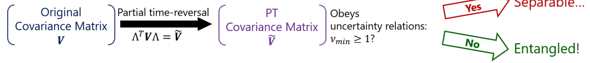
Figure 4.1: An illustration of the positive partial transpose test. Beginning with the original covariance matrix \mathbf{V} , a partial time-reversal is applied to one of the partitions, e.g. mode i of the multimode system. Then the partial time-reversed output state is checked again if it still obeys the uncertainty relations as a physicality test. If the output state is still physical, it means the subsystems in the original state, represented by \mathbf{V} , were not entangled. If the partial time-reversed matrix failed the test, it implies that the subsystems described in \mathbf{V} were entangled.
