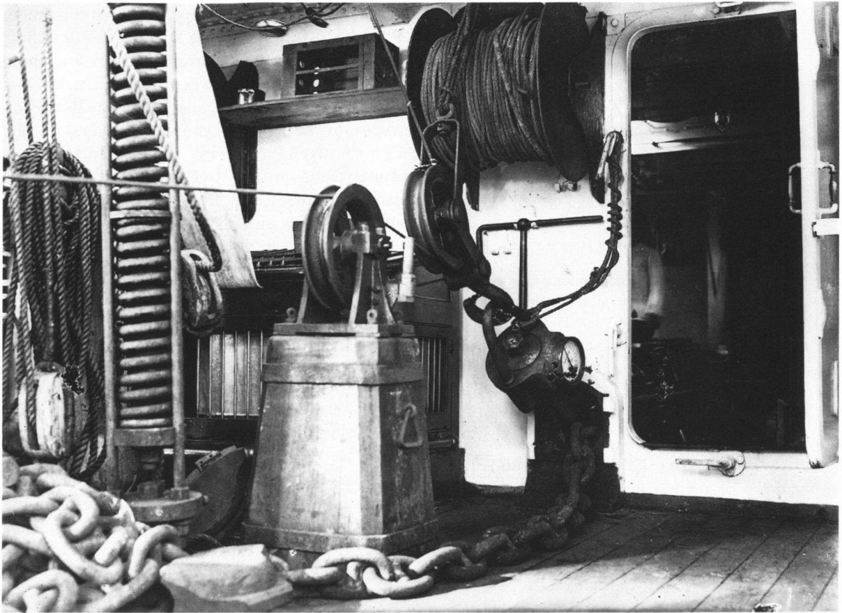
Fig. 5. View on deck of the Siboga with part of the dredging apparatus. At the left the spiral of the accumulator, in front of which the dredge rope is running horizontally over two steel blocks. The dynamometer is attached to the right steel block. At the right the entrance to the laboratory. (Cf. Weber-van Bosse, 1904: plate facing p. 2 and Tydeman, 1902b: pls. I–III.)
