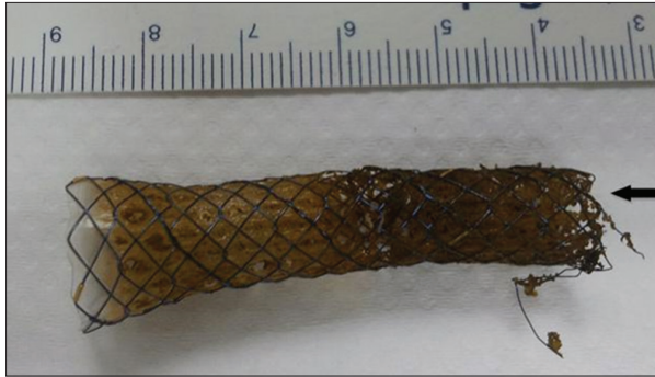
Figure 3: Fractured stent after removal. Arrow points to the fractured end of the stent
