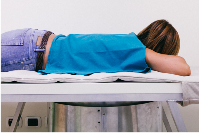
Figure 1: The microwave apparatus consists of a cup that holds the breast when the patient lies prone on the examination table. The transmitting (TX) and receiving (RX) antennas are located inside a hub and can be moved around the azimuth, to irradiate the breast (through TX) and capture the microwaves scattered by the breast itself (through RX). Both TX and RX are connected to a VNA. No matching liquid is required.
