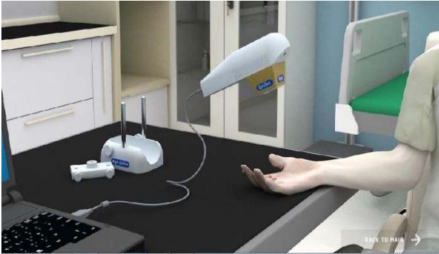
Fig. 8. Epsilon conducting a skin measurement on a patient
