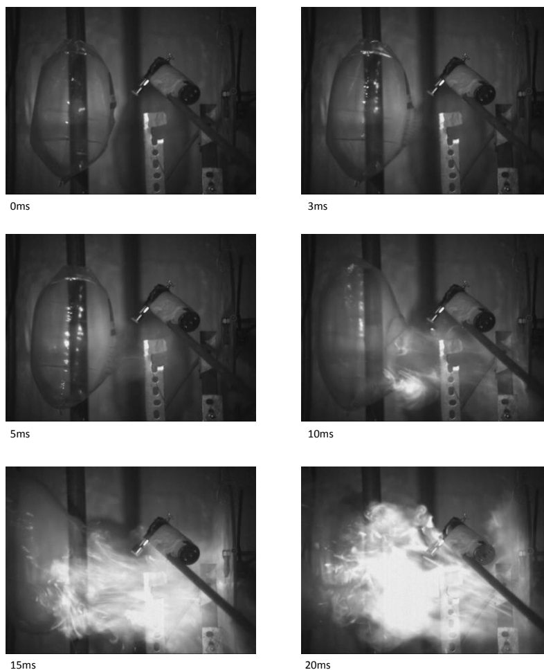
Figure 10. Image frames from ignition of stoichiometric H 2 /air mixture in a zip-tie sac with the 0.8kg pendulum.
