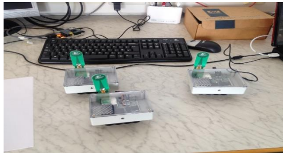
Figure 3: Three PulsOn 410 UWB sensors (each PulsOn 410 is in an enclosure).
