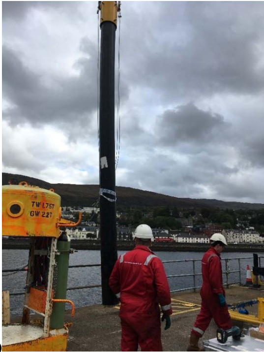
(a) Section of flexible test, 6m long and 220mm diameter, provided by TWI for the system trial. (b) Use of mobile crane to lift and lower the assembly under water.
