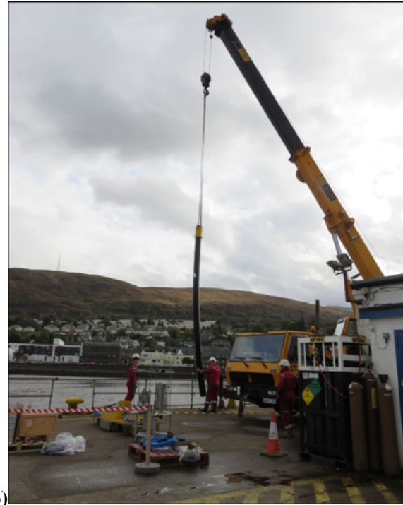
(a) Section of flexible test, 6m long and 220mm diameter, provided by TWI for the system trial. (b) Use of mobile crane to lift and lower the assembly under water.
