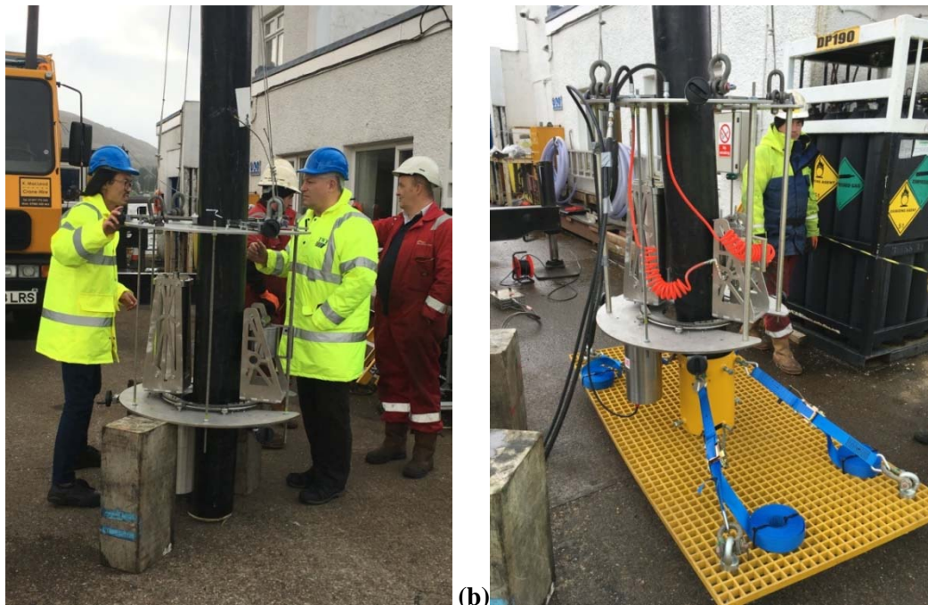
Figure 11: (a) Riser being inserted into the scanner from the top. (b) Placement of riser and assembled scanner onto mesh grating platform for seabed testing.
