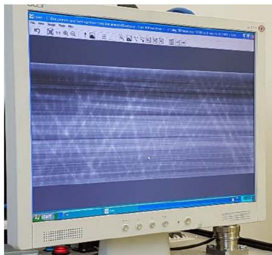
Figure 14: Live radiography image of the riser at 0.06rpm scanning rate indicating internal metal wires mesh structure of the riser.
