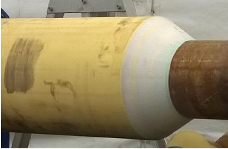
Figure 1: Linepipe coating cut back away from weld, with a chamfer included.
