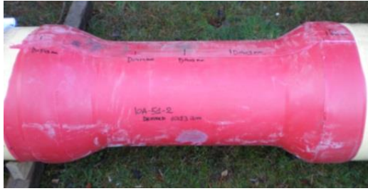
Figure 3: a) hourglass field joint coating; b) full field joint coating.
