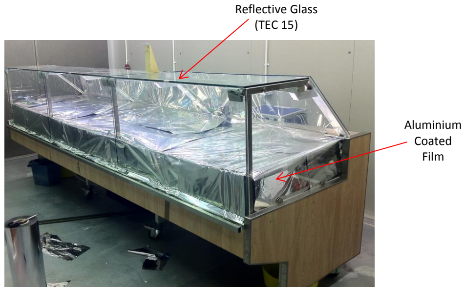
Figure 5 - Photograph showing a delicatessen cabinet with low emissivity glass and aluminium film
