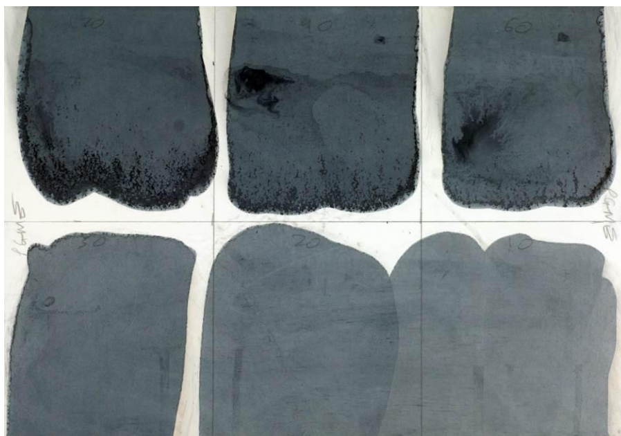
The effect of using staining times of 10, 20, 30, 60, 90 and 120 seconds for PGME-based solvent black 3 on white melamine coated chipboard.
