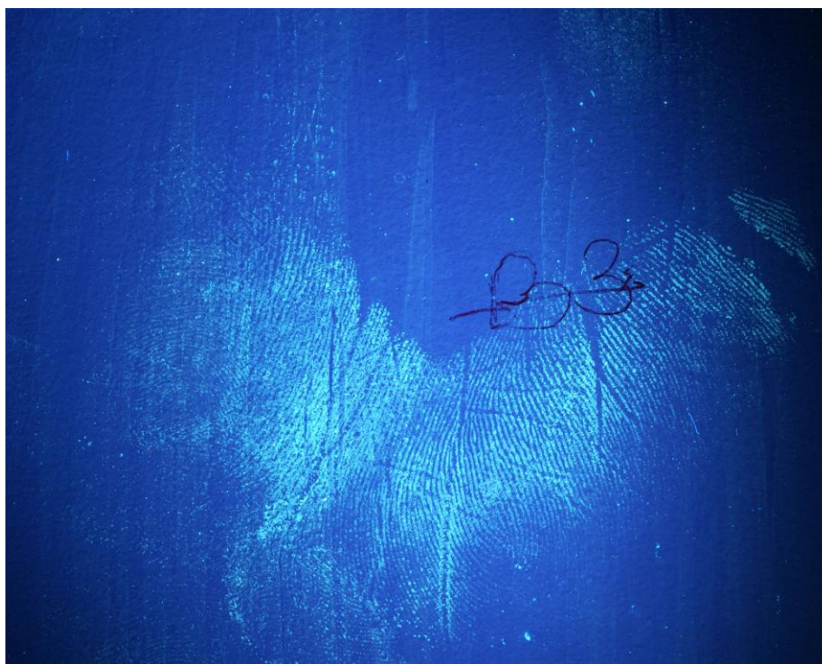
Palm mark developed on painted wall using fluorescamine.
