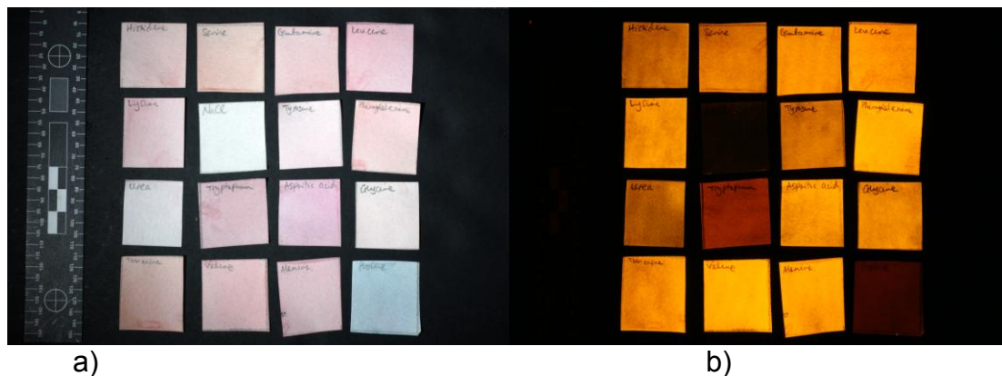
Reaction products formed between 1,8-diazafluoren-9-one (DFO) and 0.1M solutions of amino acids and other fingerprint constituents a) visible, and b) fluorescence.
