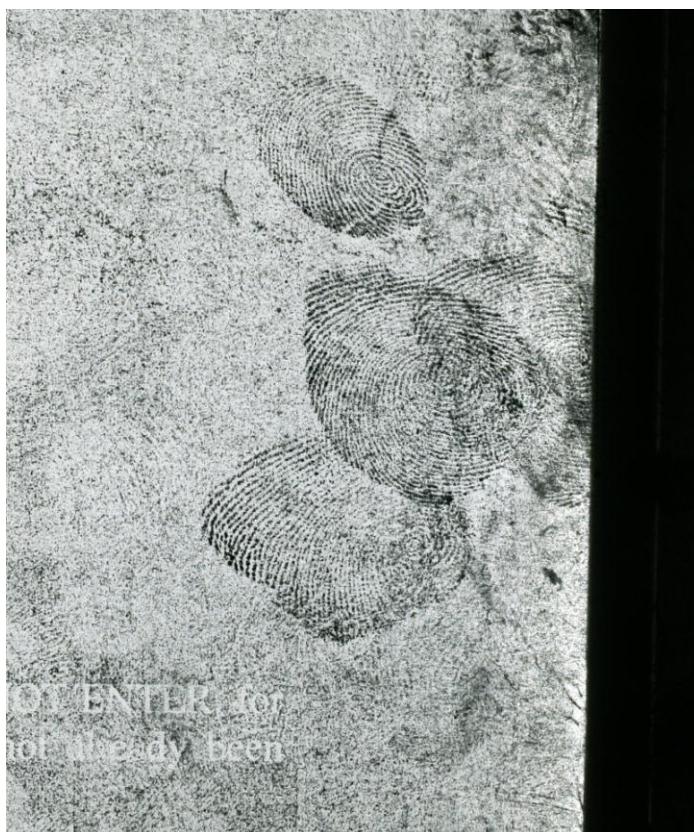
Fingermarks developed by electrostatic detection apparatus while processing a document.
