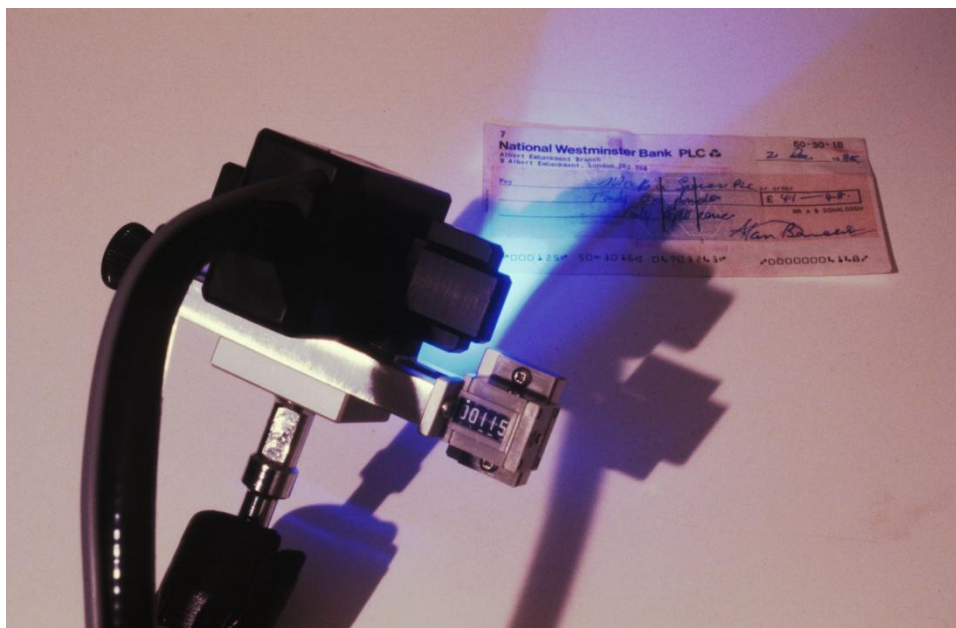
Prototype monochromator under test.
