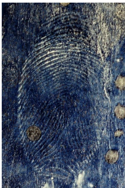
Mark deposited in a layer of Castrol grease and developed using solvent black 3.
