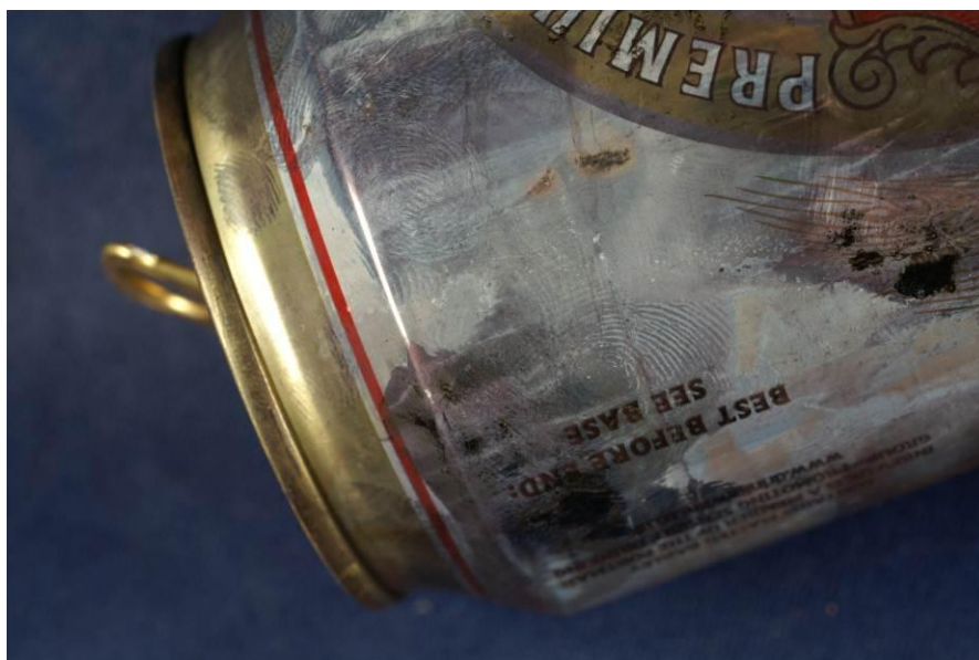
Photograph of beer can treated with solvent black 3, showing developed ridge detail.
