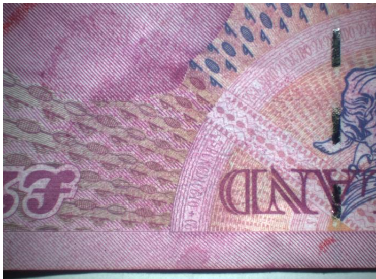
Mark developed using ninhydrin on the patterned, multicoloured background of a £20 note.
