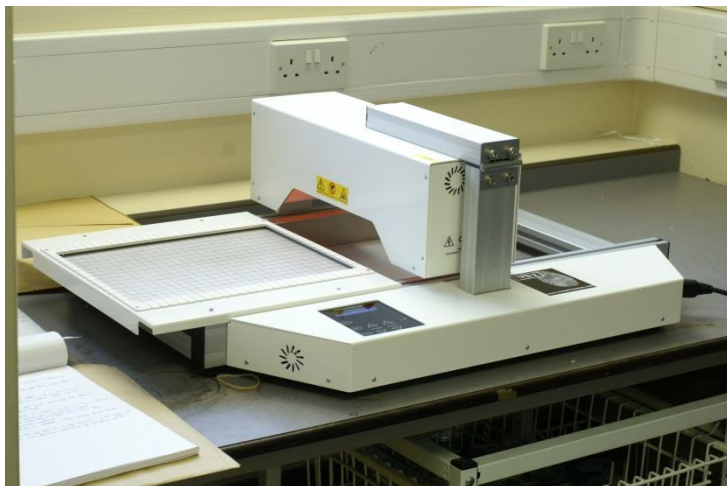
The Foster & Freeman TFD-2 system for the thermal development of fingermarks on flat paper items.
