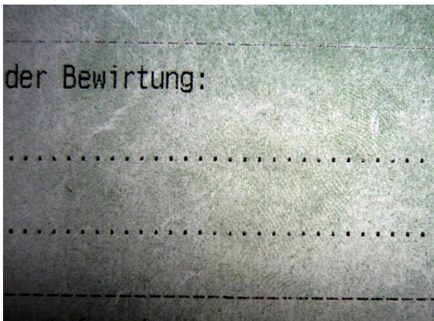
Fingermarks developed on a thermal receipt by hydrochloric acid fuming.
