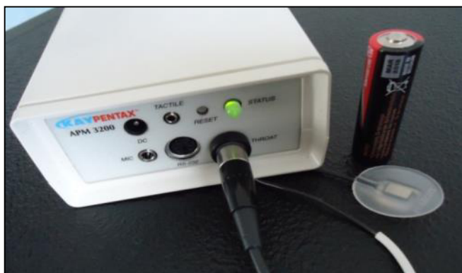
Figure 7.2: KayPENTAX 3200 APM control box and 3203 accelerometer with an AA battery for scale
