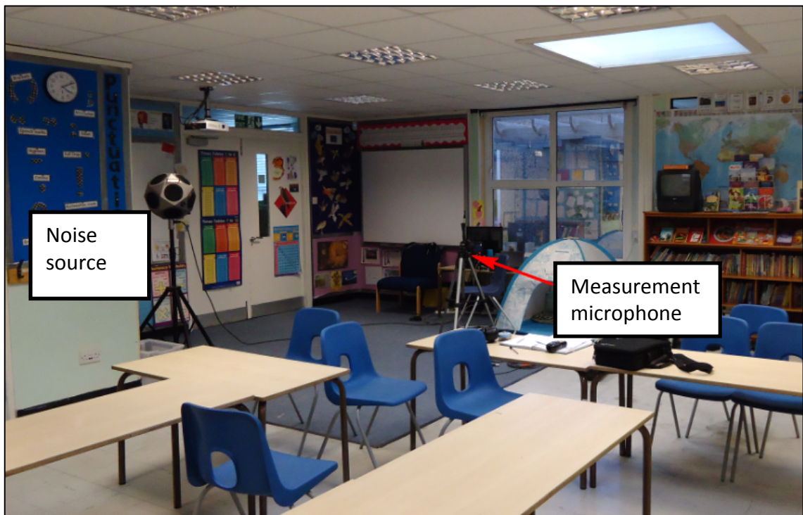
Figure 8.3: Typical arrangement for room acoustic measurements
