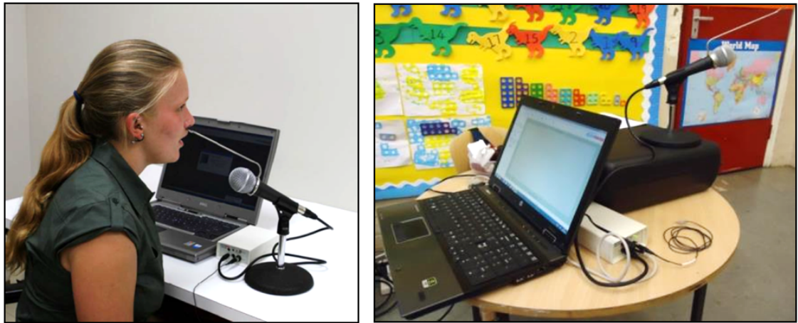
Figure 7.7: Calibration procedure using a microphone with distance guide [149]
