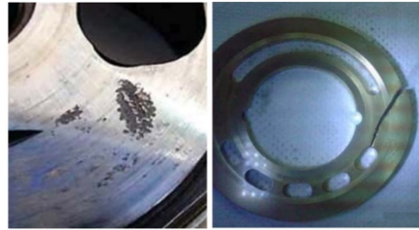
Figure 2. Compressor valve plate damage caused by corrosion (left) and fatigue (right) [24]
