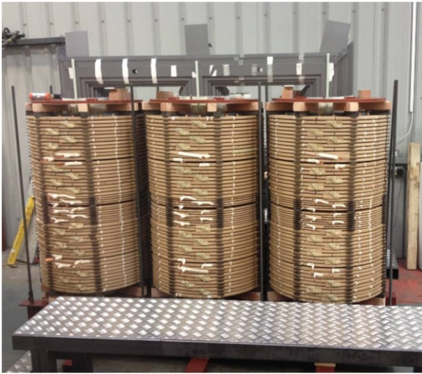
Fig. 4. Three completed (three phase) windings, high voltage (HV) discs on the outside of the core.
