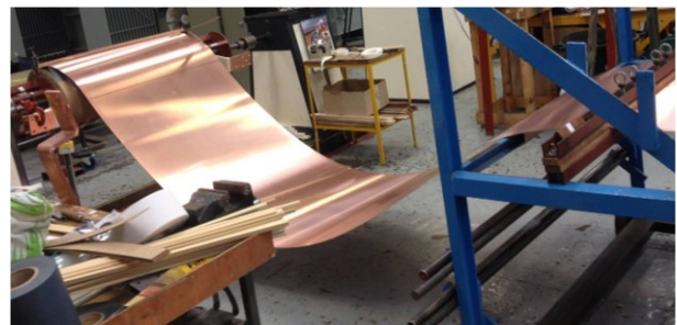
Fig. 3. The low voltage (LV) windings are usually made from wound copper foil.
