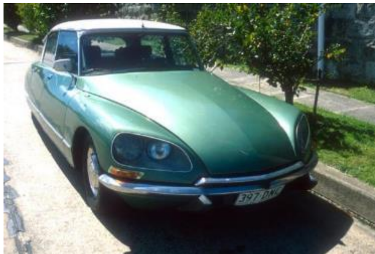
Figure A2.20 Citroën DS, probably from the mid-1970s. Here the front wings merge almost imperceptibly into the front doors – and the rear wings disappear, integrated into a full-width rear form with only a very narrow ledge on the outside of the windows.
