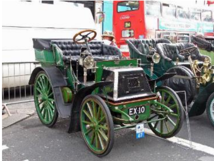
Figure A1.04 Daimler from 1900 showing a clear difference in wheel sizes. This also shows a chaincase for the final drive chain just forward of the rear mudguard and solid tyres.
