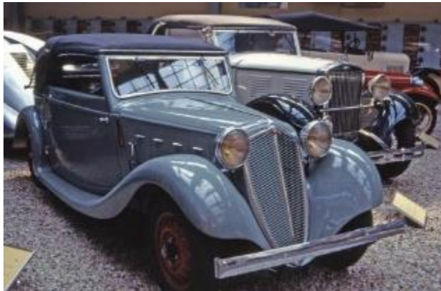
Figure A2.15 This is a car with a very short manufacturer's name – Z. It dates from 1934, and shows the flared wings starting to get the hint of valances on the outer edge, with added depth of the shaping.
