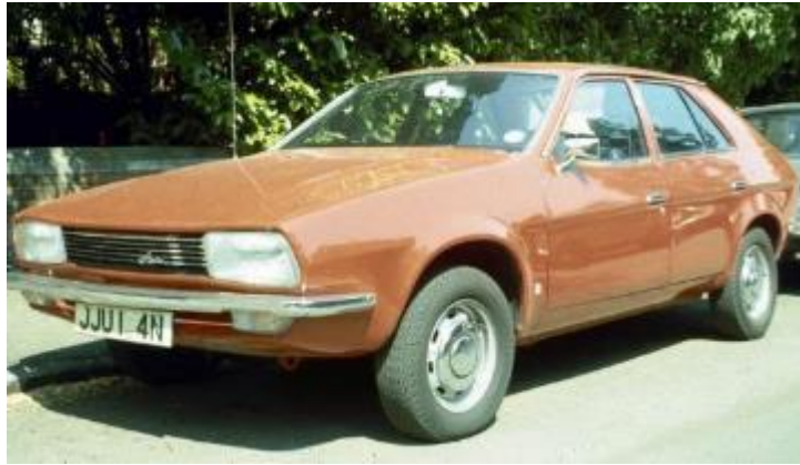
Figure A2.25 The British Leyland Princess range of the 1970s shows a clear break in the wing line at the front pillar, as does the Vauxhall Cavalier from the early 1980s (see below): (Wikimedia Commons: Charles01)
