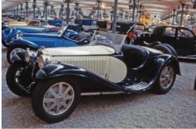
Figure A2.14 A 1932 Bugatti Type 55 showing the flowing front and rear flared wings joining each other in a smooth curving form.
