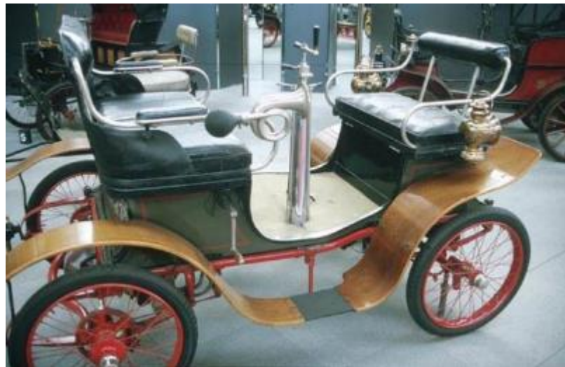
Figure A1.05 Cars without steering wheels: De Dion Bouton (1901) with a coffee grinder
