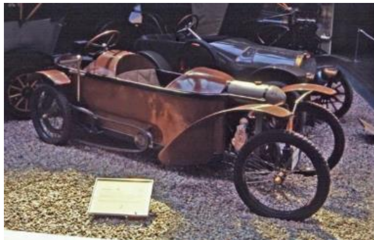
Figure A1.08 Bédélia (1913) clearly showing belt final drive
