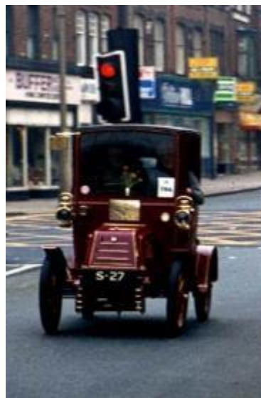
Figure A2.42 Coal scuttle with gilled tube – Georges Richard 1903
