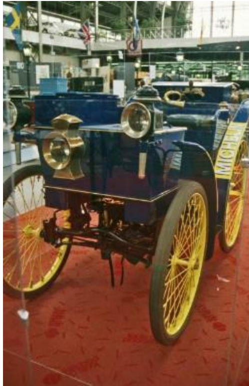
Figure 6.03 1895 Peugeot fitted with pneumatic tyres by Michelin
