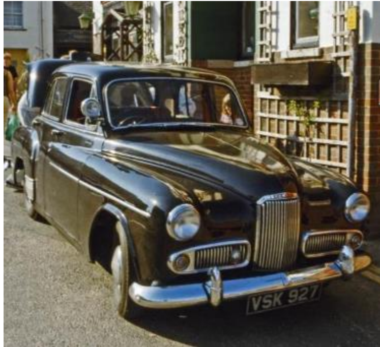
Figure A2.19 A 1955 Humber Hawk showing wings that merge with the rear wings a little higher up the body.
