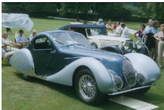
Figure A2.16 Talbot 150C, from 1939, showing valanced wings, with spats at the rear.
