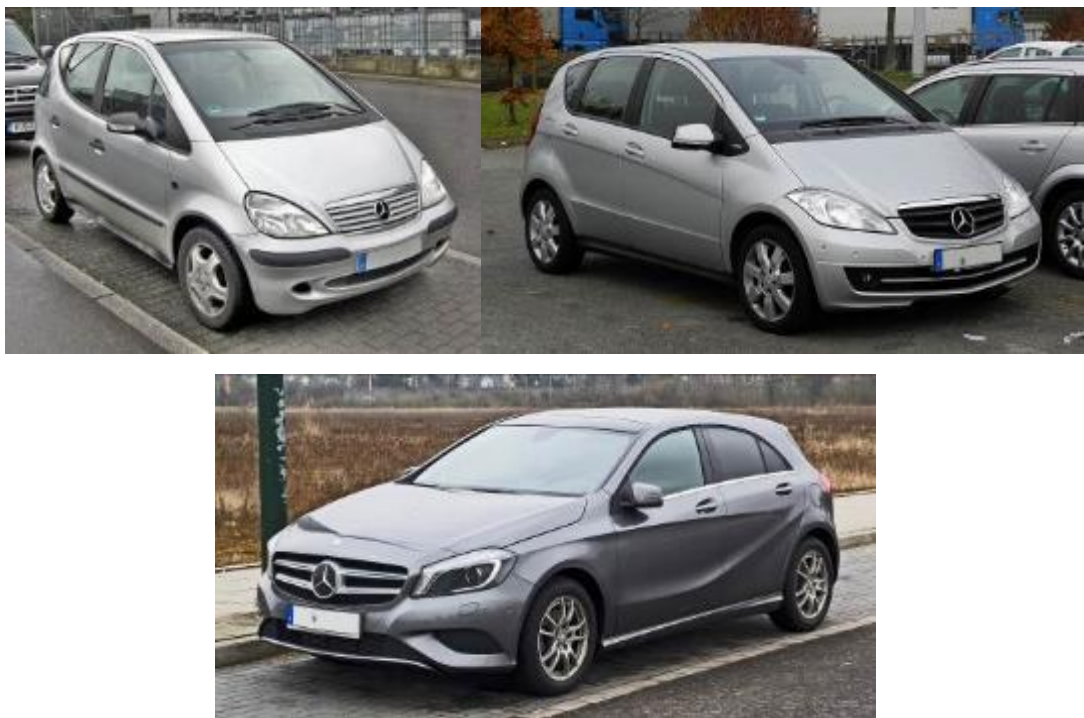
Figure A2.36 Mercedes-Benz A Class cars from 1997 – 2003, 2004 – 2012 and 2013 onwards. The lengthening bonnet can be seen, as can the 'retreat' from the two-box form that felt like an innovation when it was first introduced in 1997 (Wikimedia Commons: Matthias93).
