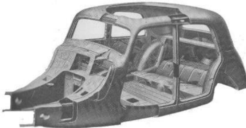
Figure 8.41 Citroën 7A body-chassis (Autocar, 1935)
