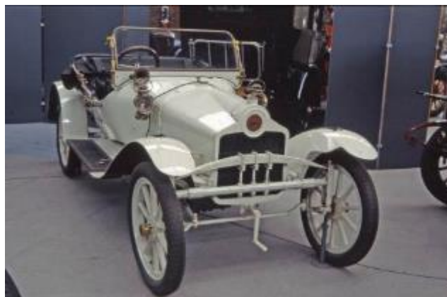
Figure A2.13 A very similar Sizaire-Naudin, but from 1910 (two years later) clearly showing the valancing behind the flared wings.
