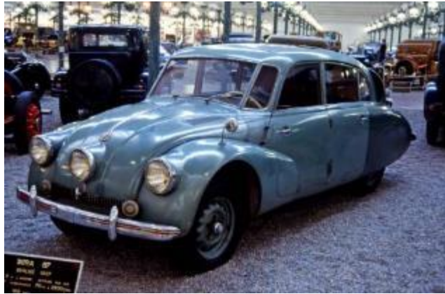
Figure A2.17 1937 Tatra 87 showing the front wings merging into a full-width body. Classic and Sports Car says that 'to think that the T87 was made at the same time as ... Western car, however, takes a considerable feat of imagination. Every detail of the Tatra stands out...' (Roberts, 2015).
