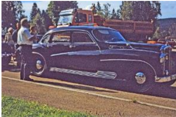
Figure A2.18 A Maybach: this is a 1938 car that was rebodied in the 1950s by Spohn. It shows the front wings flowing rearwards to join the rear wings about half way up the lower part of the body.
