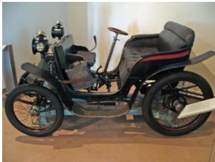
Figure 6.07 Graf, 1895. A very early example transverse-engined front-wheel drive car. This car is not part of the sample.
