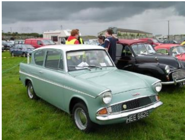
Figure A2.24 Ford Anglia showing straight-through wings with small fins at the rear. This example dates from 1967.
