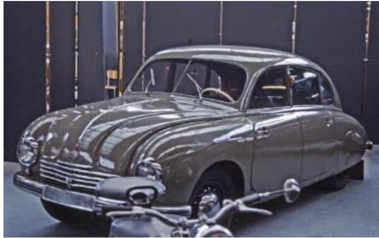
Figure A2.23 A Tatra T87 from 1951 showing a true straight-through wing lines from front to rear, also with spats at the rear.
