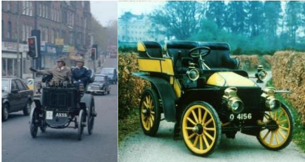
Figure A2.41 No grille – Panhard, 1892: Gilled tube – Wolseley 1901 (© British Motor Industry Heritage Trust)
