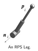
Point  $\mathbf{p}_i$  moves on plane perpendicular to  $\mathbf{n}_i$ . Point-plane constraint. Set of rigid displacements that move  $\mathbf{p}_i$  in such a way that it remains in the plane normal to  $\mathbf{n}_i$  can be expressed as a quadratic in the dual quaternions.
