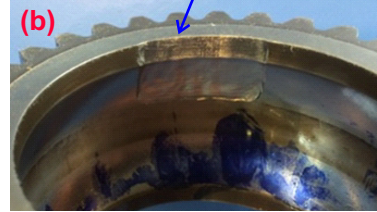
Fig. 2: (a) Second stage epicyclic gears (b) Slot across the bearing outer race; (c) Inner race natural spalling.
