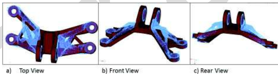
Figure 6: Overlay of Topological Optimisation on Compact Design
