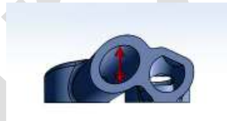
Figure 9: Section through A-A of Design I
