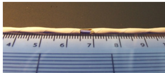
Figure 8. Defects of 5 mm hole created in the outer insulation and on the shield, on one side of the twisted shielded pair cable.
