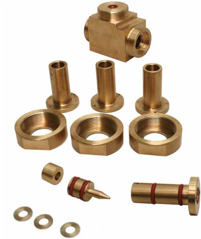
Figure 5.28: Photograph of jet-pump assembly
