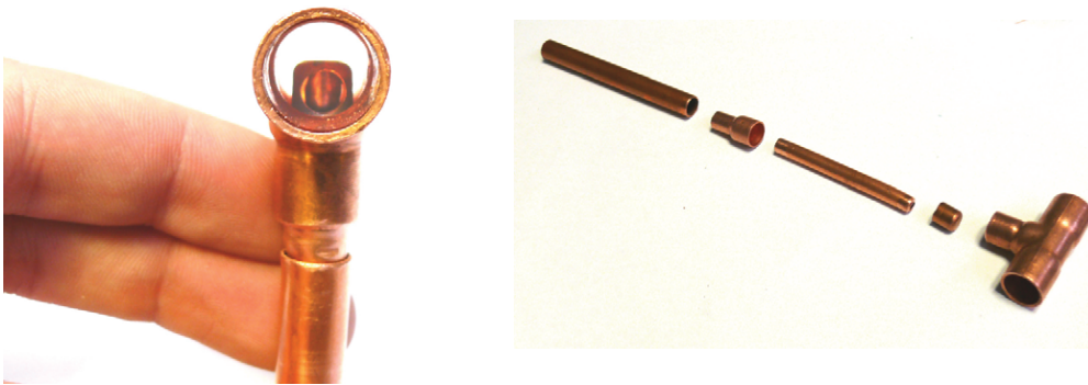
Figure 6.13: Photo - Manufacture of directional T-junction
