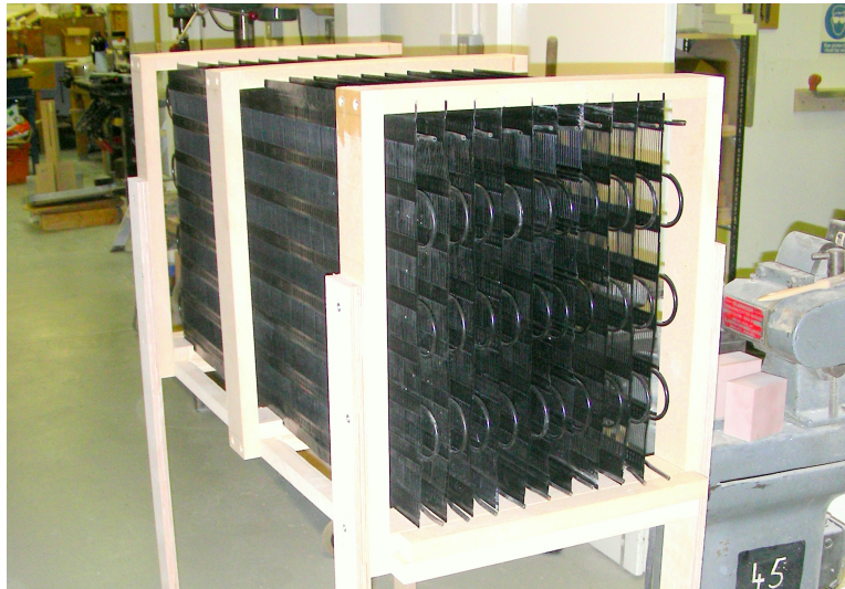
Figure 5.8: Photograph of EP1/EP2 condenser bank
