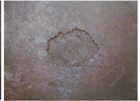
Manual tank floor inspection, underside corrosion defects
