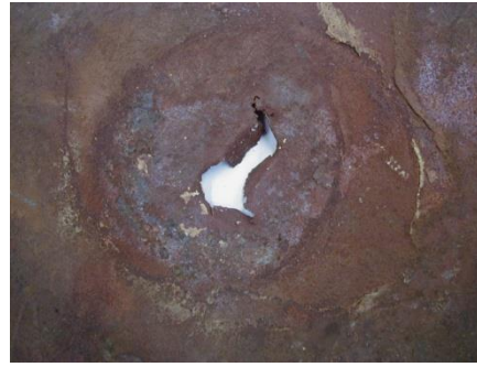
Manual tank floor inspection, underside corrosion defects
