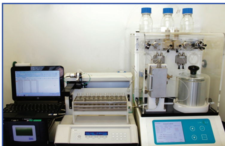
Figure 2. Continuous FlowSyn flow reactor experimental set-up.
