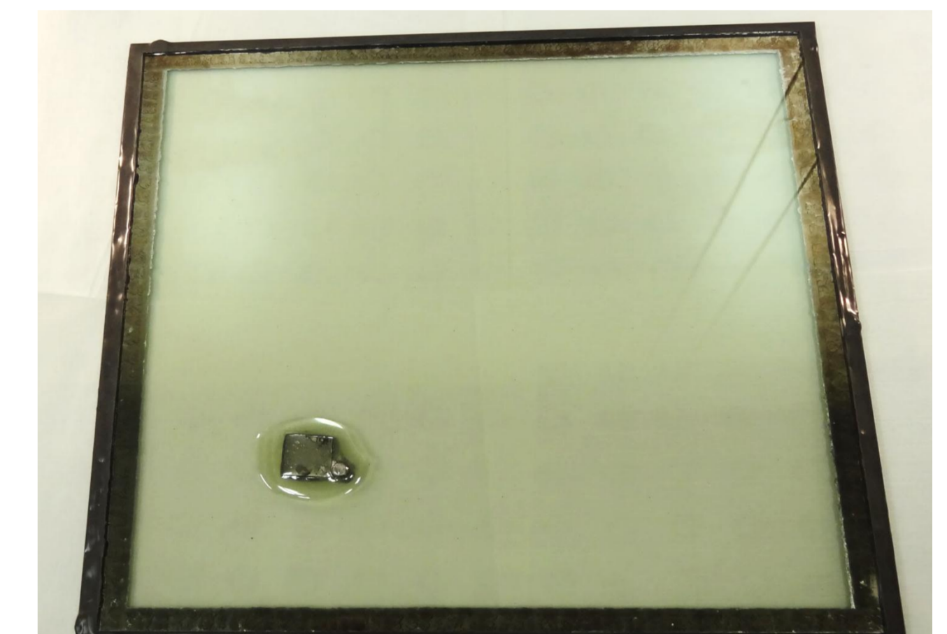
Figure 5b, Sample B, vacuum glazing 300mmx300mm achieved a pump-out pressure of up to 0.046 Pa.
