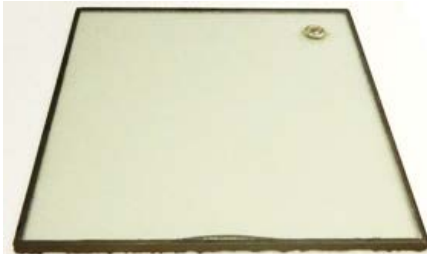
Figure 5. Sample B-400mmx400mm sample with pump-out pressure down to 0.1 Pa.
