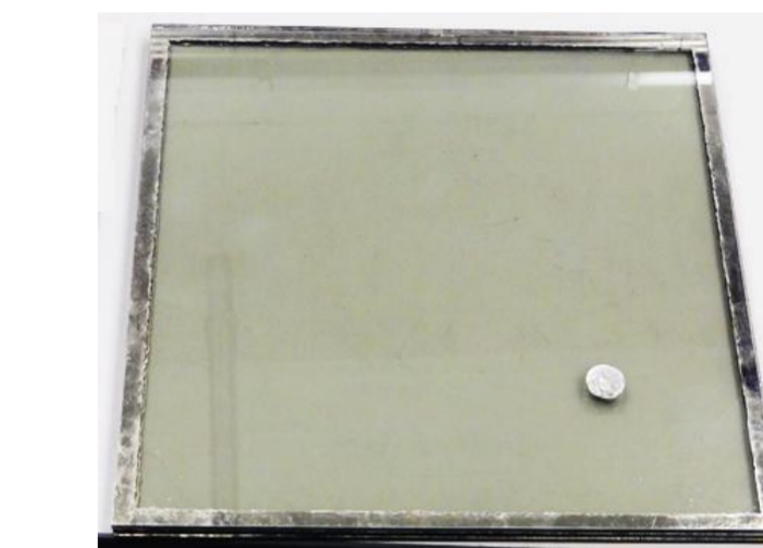
Figure 4: 0.3mx0.3m sample of Triple vacuum glazing using indium as sealing material
