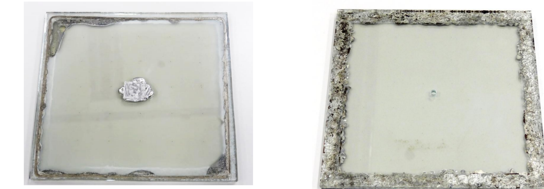
Figure 3: A cost effective Glass/Metallic sealing material for the fabrication of vacuum glazing
